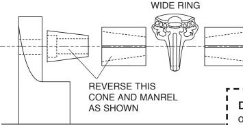
**DO NOT OVERTIGHTEN -** Damage may occur to the ring being held.
